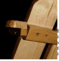
Finally, put a screw through the small lump of wood under the armrest into the upper back support. All that is then needed is to cut a small shaped piece of wood to support the front of the arm rest (where it meets the front leg) -- thus stopping it from bending when pressure is placed on it.
